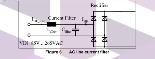
The required  $L_{\text{filter}}$  is:
