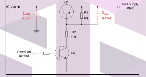
Figure 20 Vcc supply circuitry
