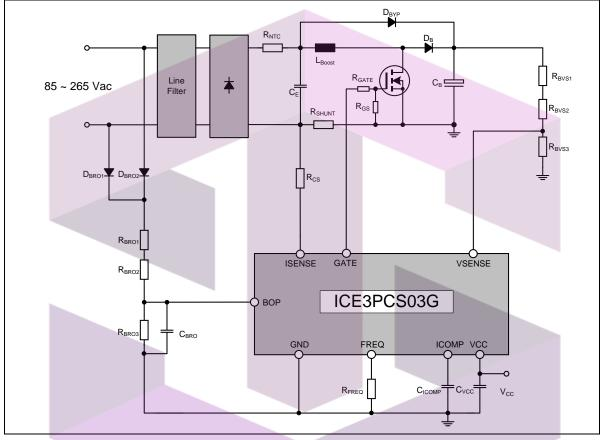
Figure 4 Typical application circuit of ICE3PCS03G
